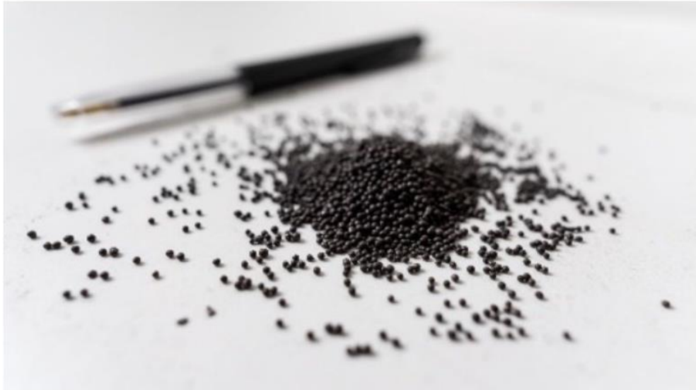
Figure 5: The spherical steel shot particles - diameter 0.6 to 1.2 mm. Picture by Tessa Veldhorst De Schaapjesfabriek©.
